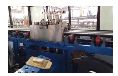
The Bar test systems is to test the defcets Longitudianally oriented defects based on the International Standard. The Test Mechnism will have Immersion tank having various probes for the longitudinal oriented defects.
